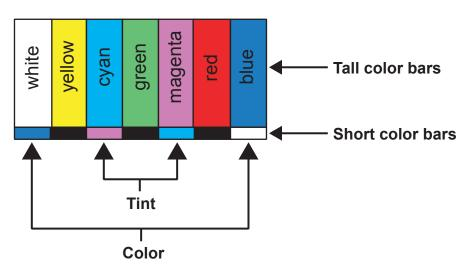
**TINT** (also known as 'hue') is essentially the ratio of red to green in the color portion of the image. If TINT is decreased, the image will appear redder, and increasing it will cause the image to appear greener. To set TINT properly, look at the color bar pattern through a blue filter (or mute the red and green outputs). Adjust TINT until the middle two tall color bars match the middle short color bars (see color bar drawing).
